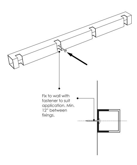
2) Fix support extrusions in parallel - Fit off blades temporarily to accurately position fixing extrusion.
