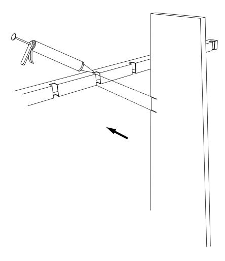
4) Fix blades off starting from the center. Wipe away excess silicone with a damp cloth.
