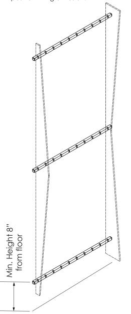
Appy Liquid Nails General Purpose to inside of extrusion prior to fixing the blades.
